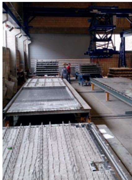
Afterwards: Demoulding at two pallet positions and three destacking stations and two run-off carriages
