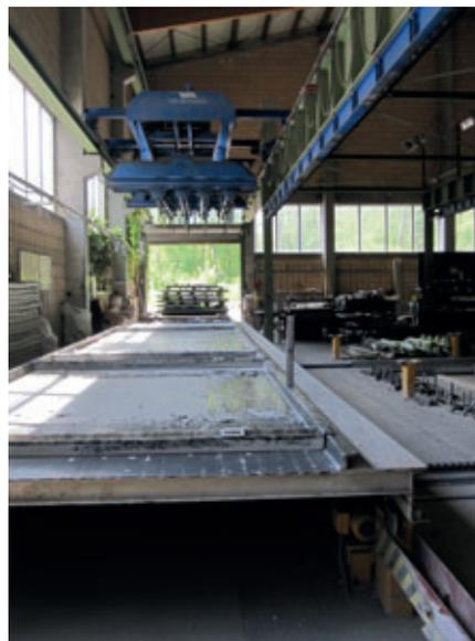
Previously: Demoulding at only one pallet position and only one destacking station / run-off carriage
