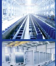
**CASTING BEDS** are perfectly suited to produce prestressed floor slabs economically and efficiently. The consistent design and **individual optimisation of the production lines** are the alpha and omega in this regard. Our support for our customers already starts with the planning stage to ensure efficient processes all the way from concrete supply to loading for transport.
