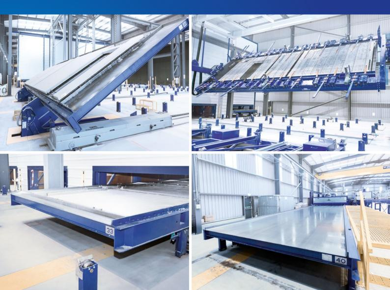
PALLET TRANSPORTATION to transport the pallets within the circulation system, the transportation technology at Weckenmann comprises the complete range of individual handling technologies. Depending on the design of the material flow concept, individual workstations are networked through friction wheels, cross lifting trucks, central transfer tables, central sliding stages or by a combination of these components.
